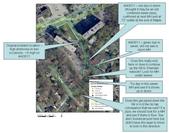
Figure 14. Stormdrain investigation of manhole KE02.
