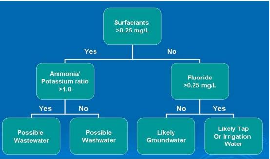
Figure 6. Flow chart method used to distinguish potential illicit discharges (Brown et al, 2004).
