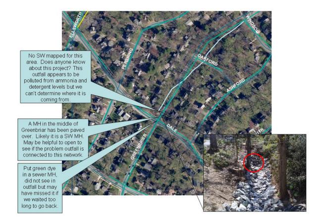
Figure 16. Outfall at Dale and Greenbrier circled in red.
